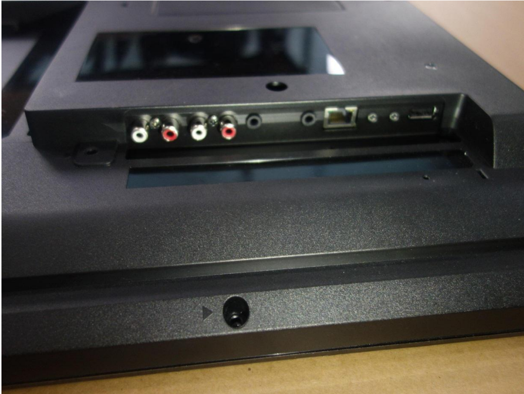
Figure 7. Data ports on main board
