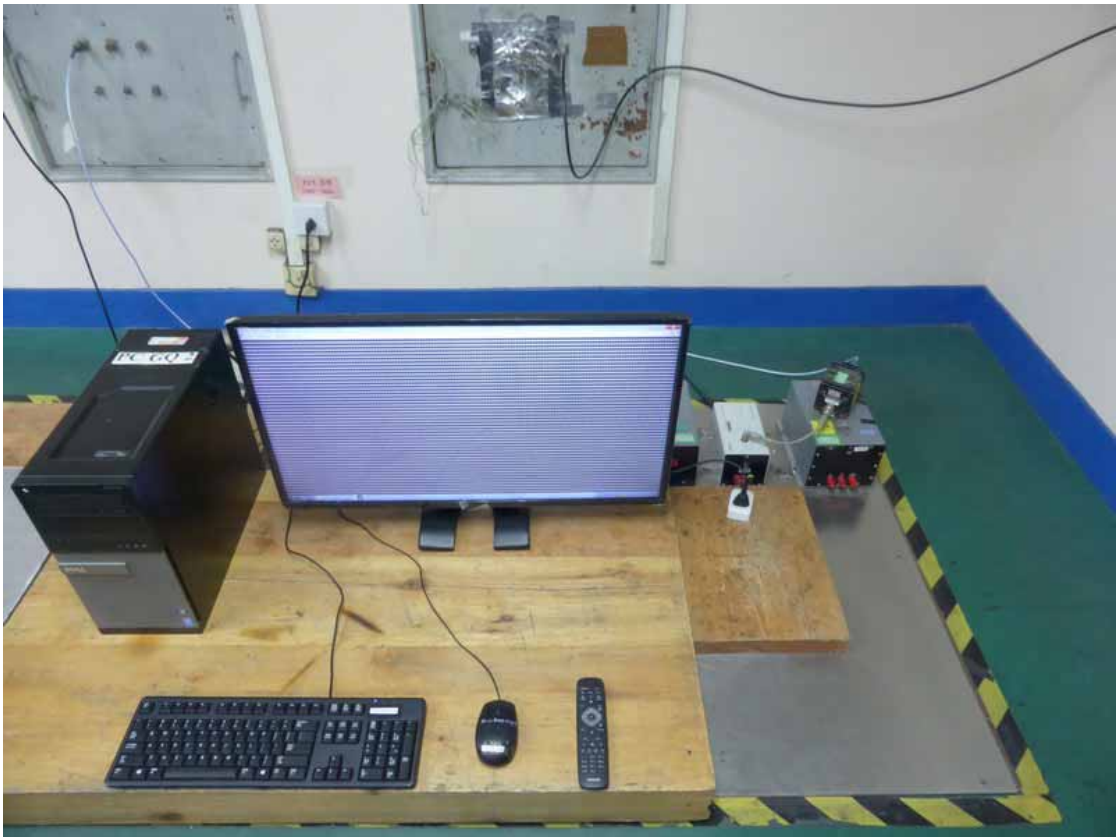
16.9. Photo of Injected Currents Susceptibility Test
