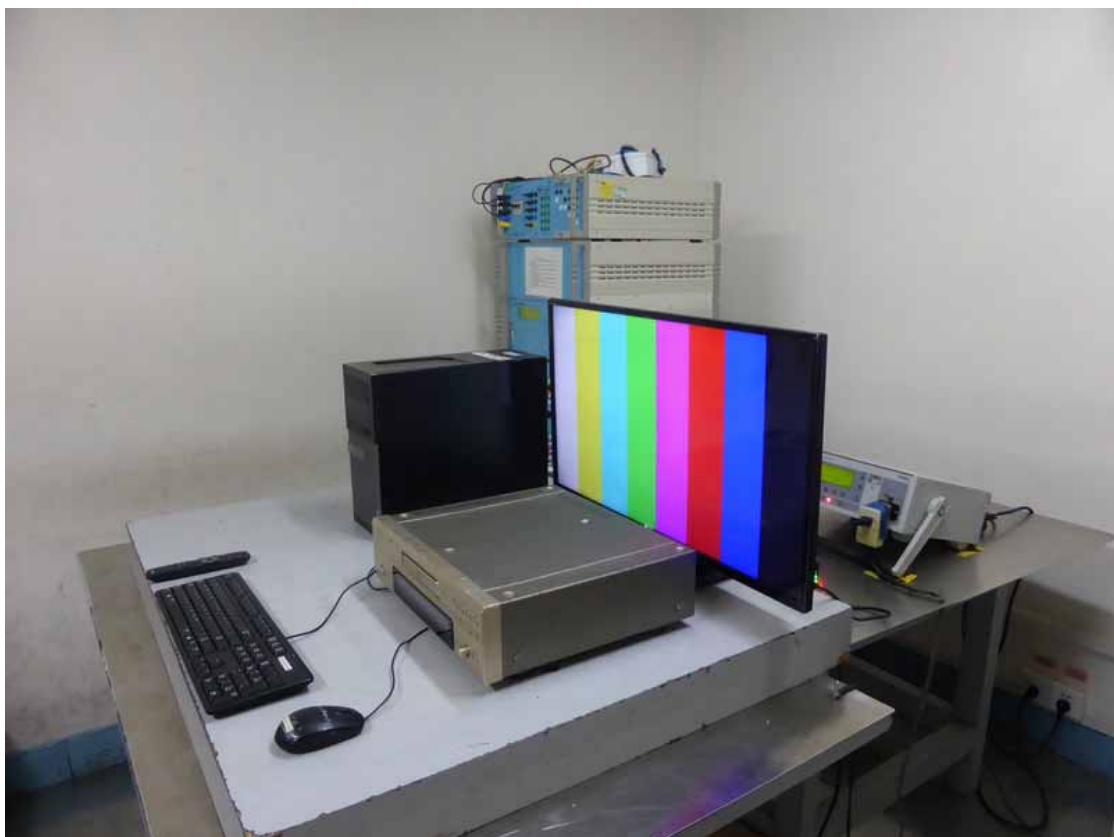
13.6. Photo of Electrical Fast Transient/Burst Immunity Test
