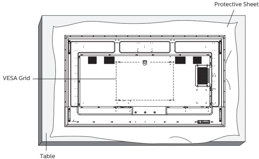
1. Spread a protective sheet which was wrapped around the display when it was packed on a flat surface. Lay the display face-down on the protective sheet to facilitate your operation without scratching the screen.
