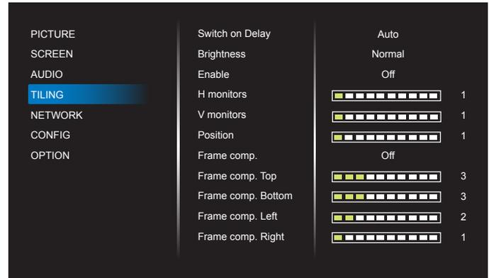
With this function you can create a single large-screen matrix (video wall) that consists of up to 150 sets of this display (up to 10-sets on the vertical and 15-sets on the horizontal sides). This function requires an external splitter or controller.
